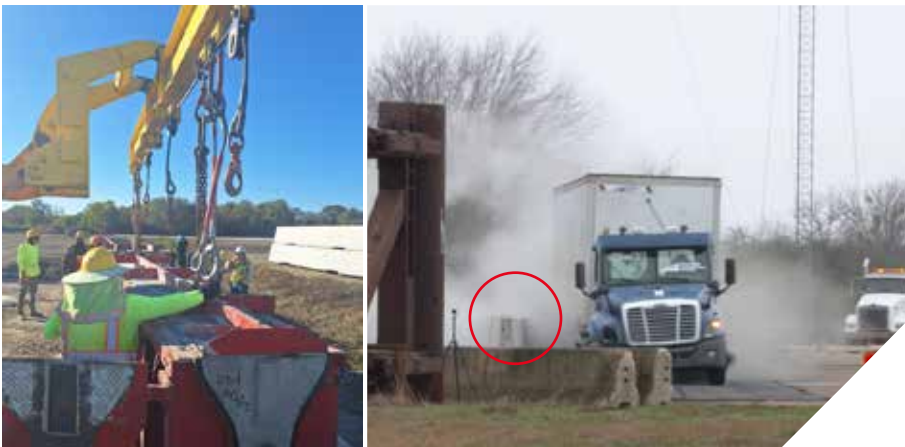
Mobile production and crash testing in Texas: the DB 120 also copes well with US HGVs.
